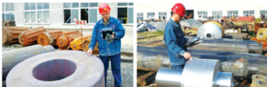
探伤质量检查 Ultrasonic Examination
